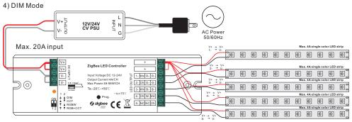
Note: please make sure the dial switches are at position for DIM mode as shown in above diagram
