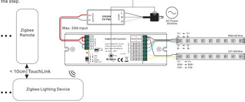
Step 2: Set another device or remote or touch panel into network pairing mode and pair to the network, refer to
