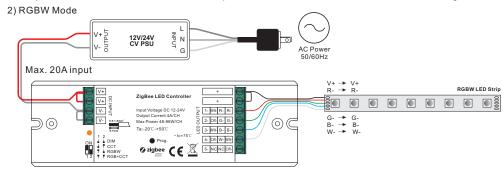
Note: please make sure the dial switches are at position for RGBW mode as shown in above diagram.
